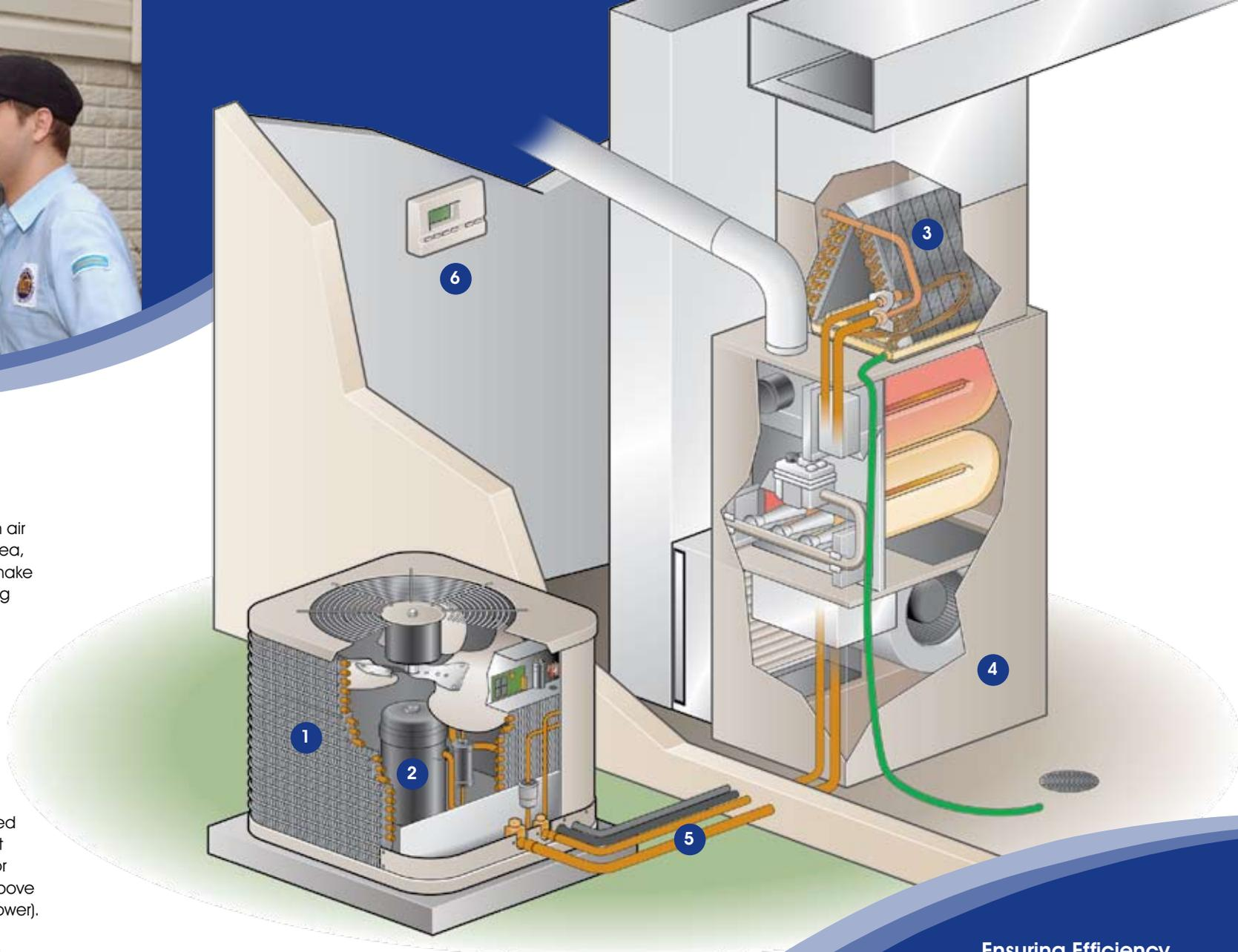
The cycle continues until the room reaches a set temperature on a **thermostat (6)**. When the thermostat senses that the room has reached the set temperature, it turns off the air conditioner. As the room warms up, the thermostat turns the air conditioner back on.
